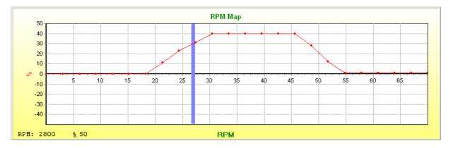
With these 2 graphs the cams can be manipulated with RPM and engine load.
